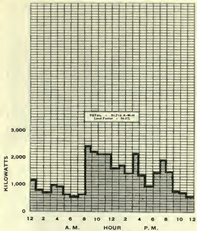
FIG. 615. ENERGY CHART. Kilowatt-Hours at the Pantograph for the Average October Day for 2,400-Volt D. C. Operation, Freight Transfer Service on the C. & N. W. Ry.
